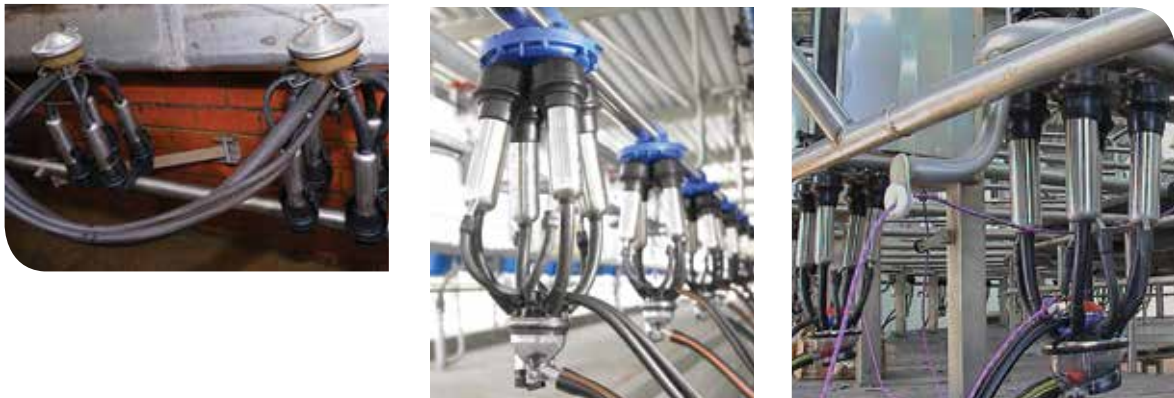
Figure 9 Clusters attached to jetters mounted on the jetter line in the cleaning position (example only). Two different cluster orientations when attached to the jetters are shown
