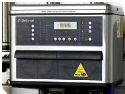
Figure 4 Automatic wash controller for milking machines (example only)
