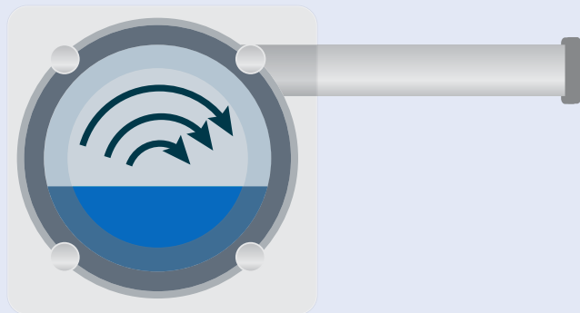
Figure 40 A well-formed slug can create good turbulence (swirling action) and effective cleaning in the receiver
