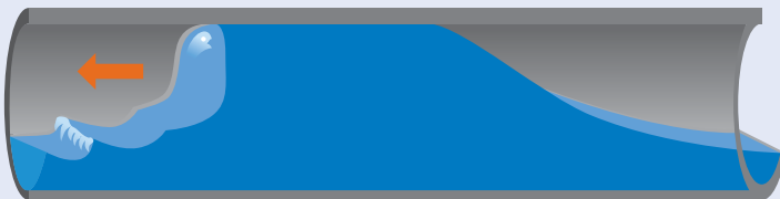
Figure 38 A well-formed slug in the milk line
