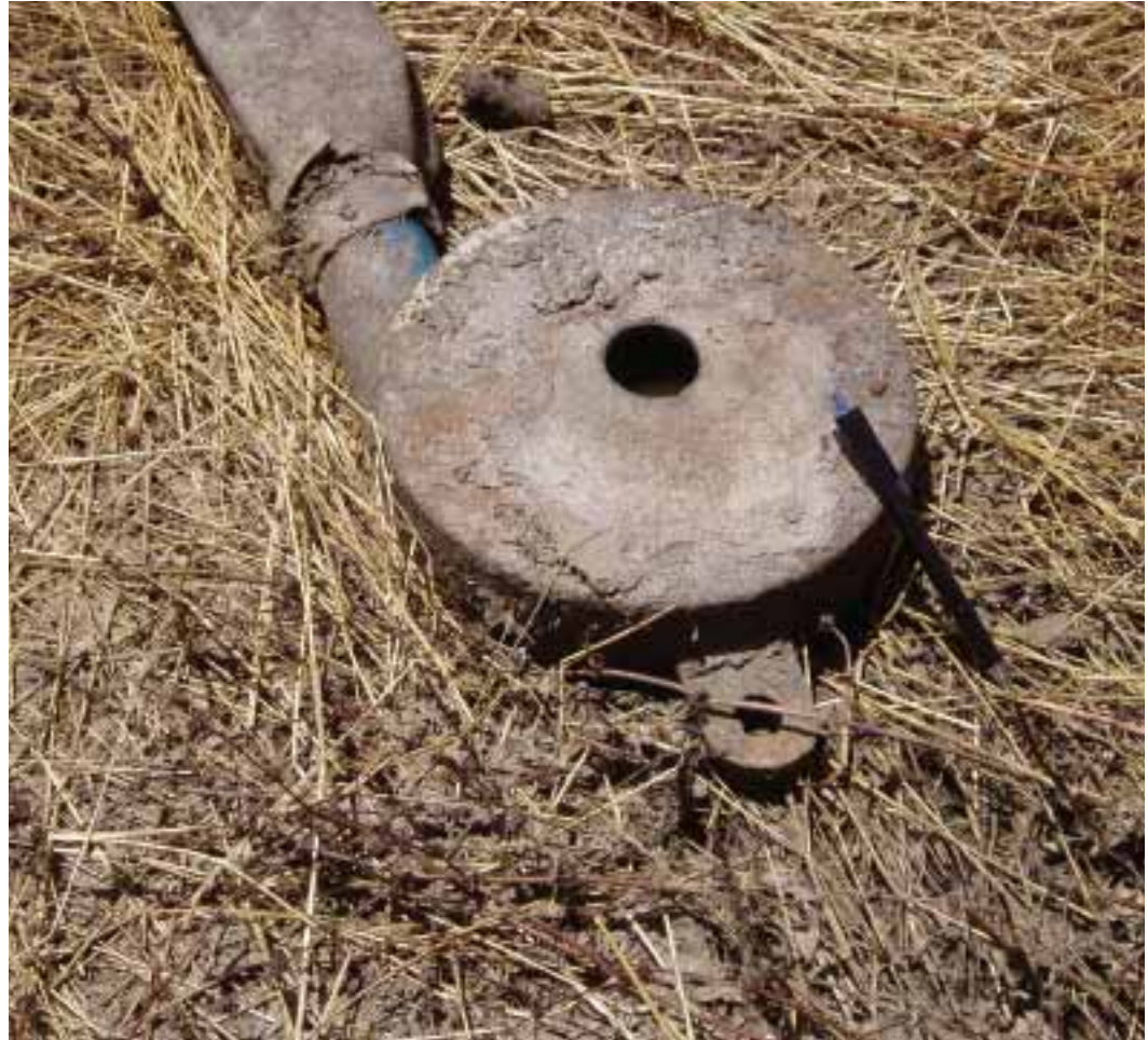
FIGURE 6.15. Stationary pot sprayers have to be moved around manually on a daily basis
