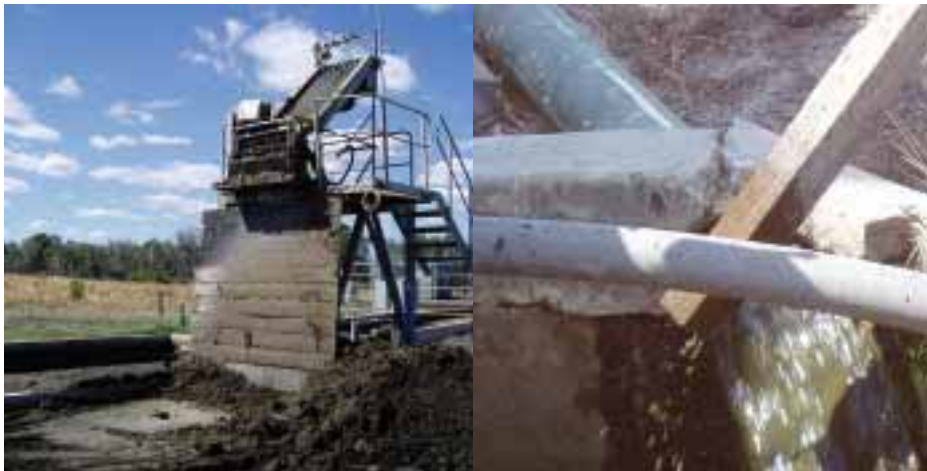
Solid separation device produces liquid ready for reticulation onto pastures at the Bell dairy
