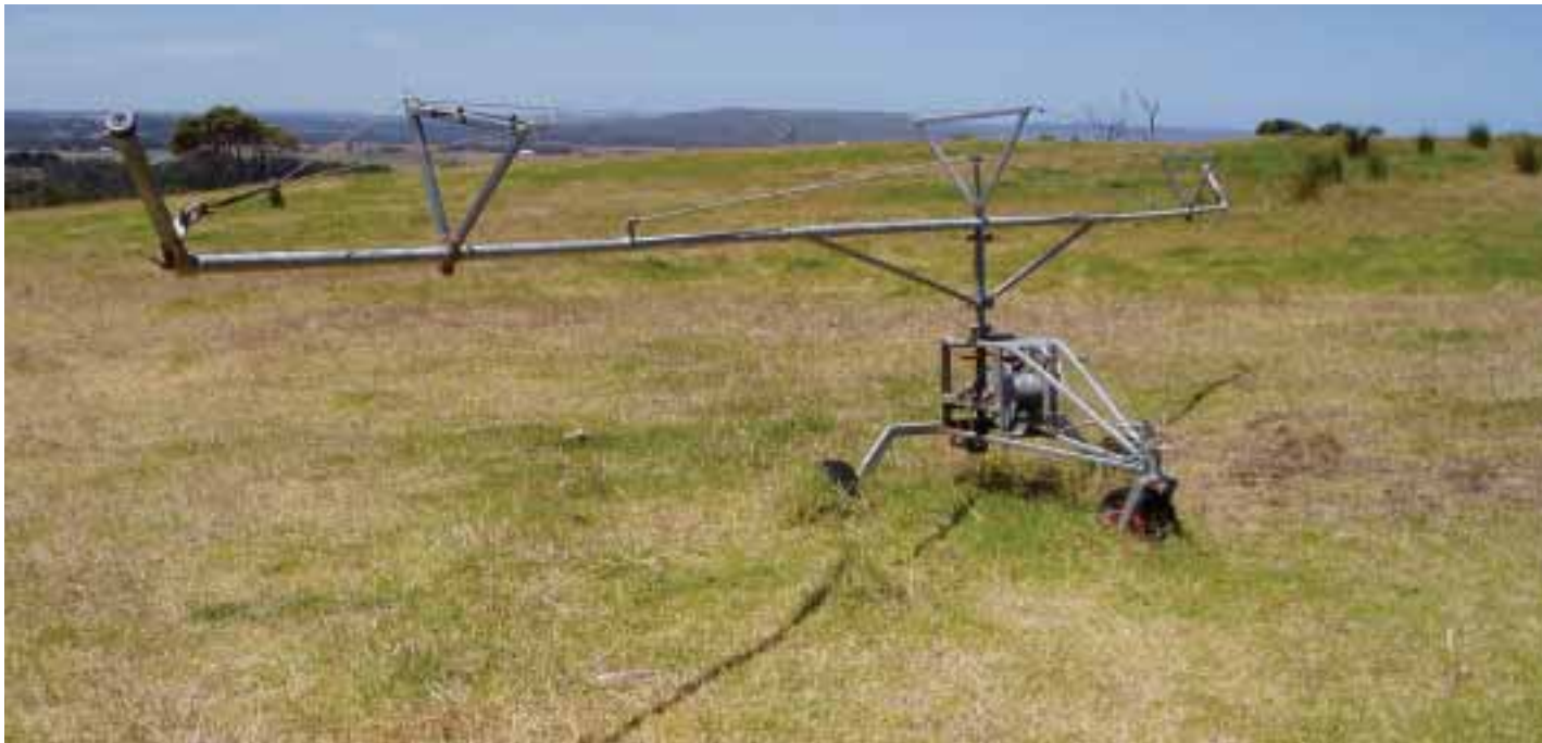
FIGURE 6.11. Self-propelled travelling rotating arm irrigator
