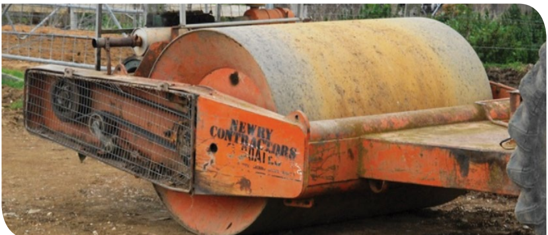
Vibrating roller for compacting laneway during construction of base layer
