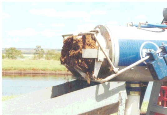
Press Screw with Solids Extruding
