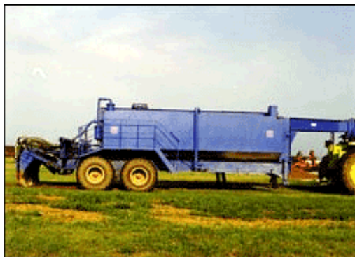
Sludge Injection Tanker
