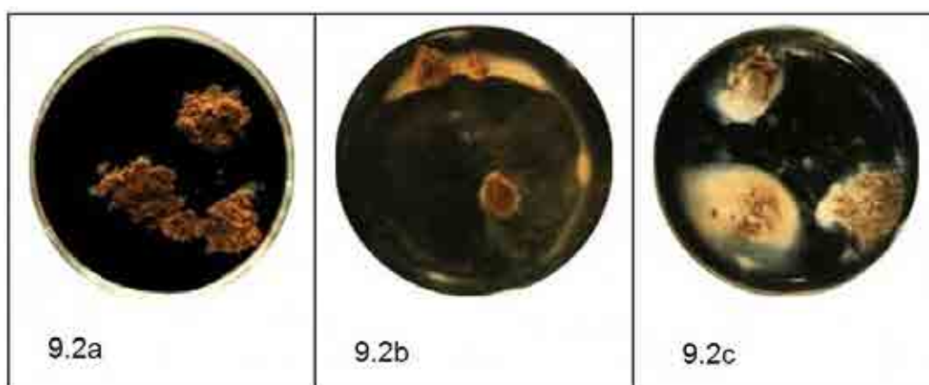
Figure 9.2 The photographs above show the results of soils placed in dishes of distilled water after a period of time. Figure 9.2a shows small clods of soil which have slaked only, Figure 9.2b shows dispersion only, and Figure 9.2c shows both slaking and dispersion (Retrieved: http://vro.dpi.vic.gov.au/dpi/vro/vrosite.nsf/pages/soil_mgmt_slaking . Images by Stuart Boucher).
