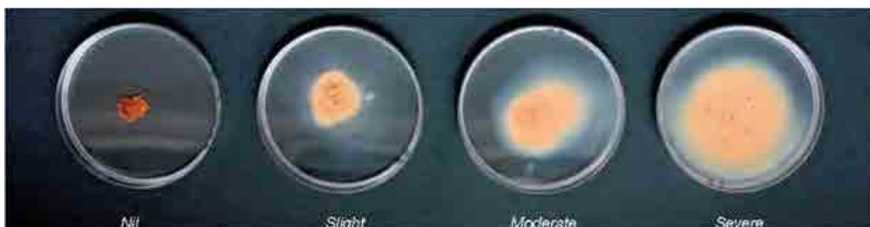
Figure 7.3 Increasing levels of soil dispersion, from left to right, when dispersion is determined using deionised water. Source: http://www.agric.wa.gov.au/PC_93842.html
