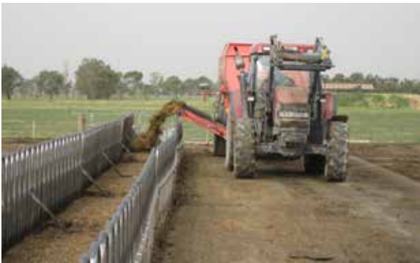
Silage fed out with silage cart into low-cost troughs ('Waste-Not Fair Go Dairy Feedpad' panels)
