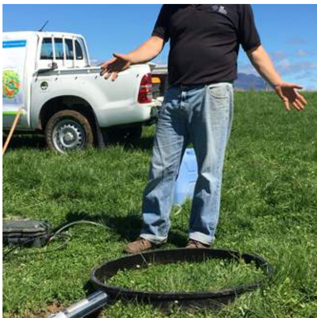
Figure 3b Soil infiltration testing
