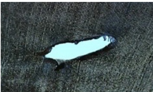
Damage to shade cloth caused by tractor exhaust. This shade cloth structure is only 3.5m high. Shade structures should be ideally at least 4m
