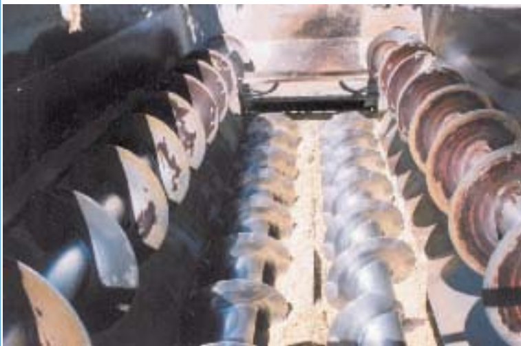
Internal auger system of a mixer wagon.
