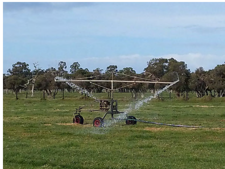
Traveling irrigators are a cost effective method to reuse effluent Photo credit: GeoCatch
